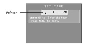
If the control panel is not set at the current time, use the left arrow to go back over the columns and the up arrow to make changes.
